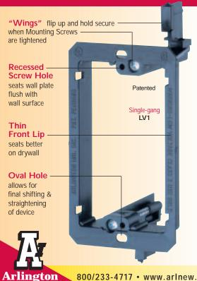
Use Arlington's non-metallic mounting brackets to install class 2 wiring - and to seat wall plates flush with the mounting surface.
