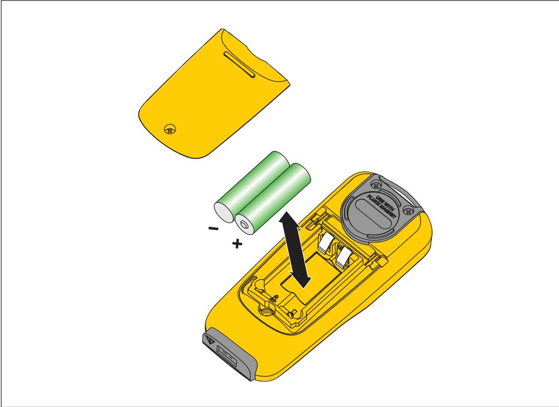
**Figure 4. Battery Replacement**
