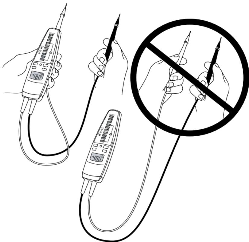
Figure 5. Rotary Field Measurement
