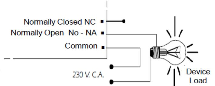
**CONSIDERATIONS ON THE OUTPUT.** During the operating mode and according to its load, may fluctuate or malfunction output. If this happens, install a circuit spark between the two relay contacts used in connection as shown in the drawing.
