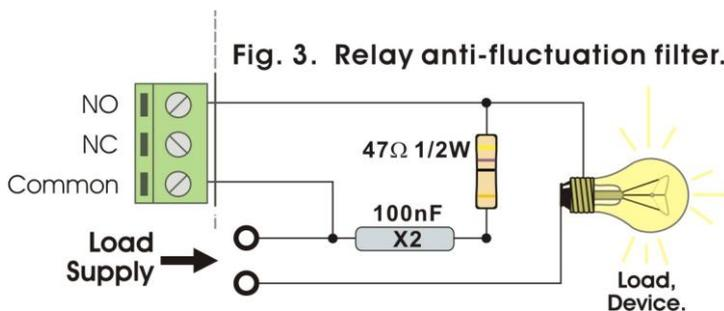
**Note:** To connect load at 12V DC, you have to remove the resistor and to only use the capacitor.
