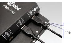
Use these holes to secure the HDMI cables with a cable tie.
