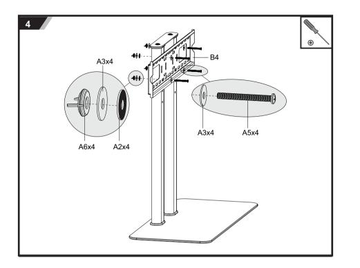
Determine the optimum height on the rear pedestal to attached the (B4) bracket. The best method to do this is to measure from the center of your television screen to the bottom most edge of the TV set. This will tell you the minimum clearance needed on this Universal Base.
