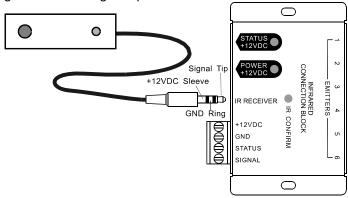
**System Connection:** Connect the IR system to the detachable connector labled +12VDC, GND, STATUS, and SIGNAL.
