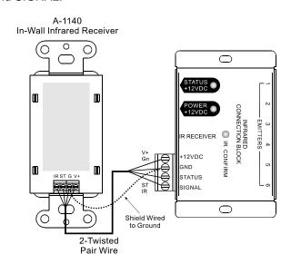
**Emitter Outputs:** Connect up to 6 emitters (A-1141 or A-1142) to the emitter jacks labeled 1-6. Place the emitters on the source equipment.
