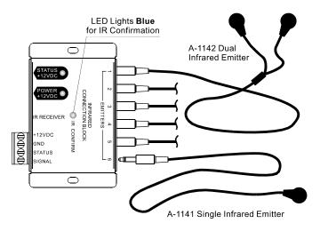
**IR Confirm:** When an IR signal is received the IR confirmation blue LED will flash.
