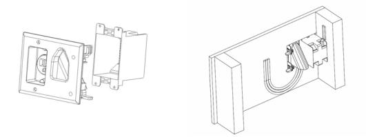
Once you have wired the receptacle, begin by inserting receptacle portion of the plate into the retrofit work box. Once the entire recessed plate is flush to the wall, using the two white screws supplied, screw the receptacle portion of the plate to the work box. **INSTRUCTIONS ARE CONTINUED ON THE BACK SIDE OF THIS PAGE**
