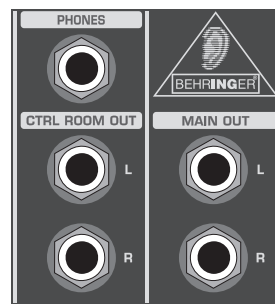
Fig. 2.9: Monitor/main mix connectors
