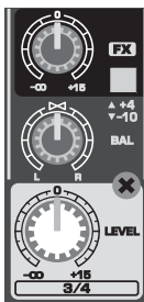
Fig. 2.6: The FX send/balance/level controls
