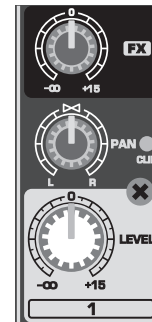
Fig. 2.3: The FX send/panorama/level controls
