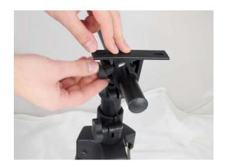
3. Repeat this process for the next support bracket. Snap it on to the other side of the tbar. When reinserting the knob, make sure not to tighten too much, as you'll need to adjust their position to line up with the laptop plate.
