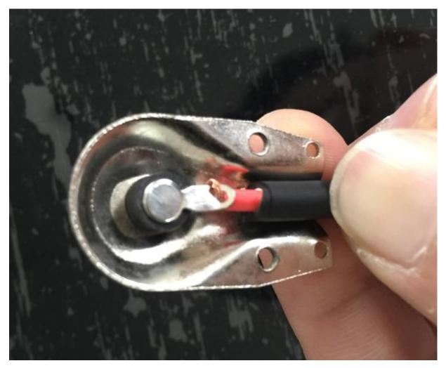
Screw the front shell on ,be careful that the black outer jacket not turn around otherwise the shielding wire will lose the contact with the body. Please screw tightly.
