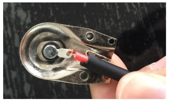
Press the main wire down a little in order to prevent it from touching with the front shell otherwise it will be short circuit.
