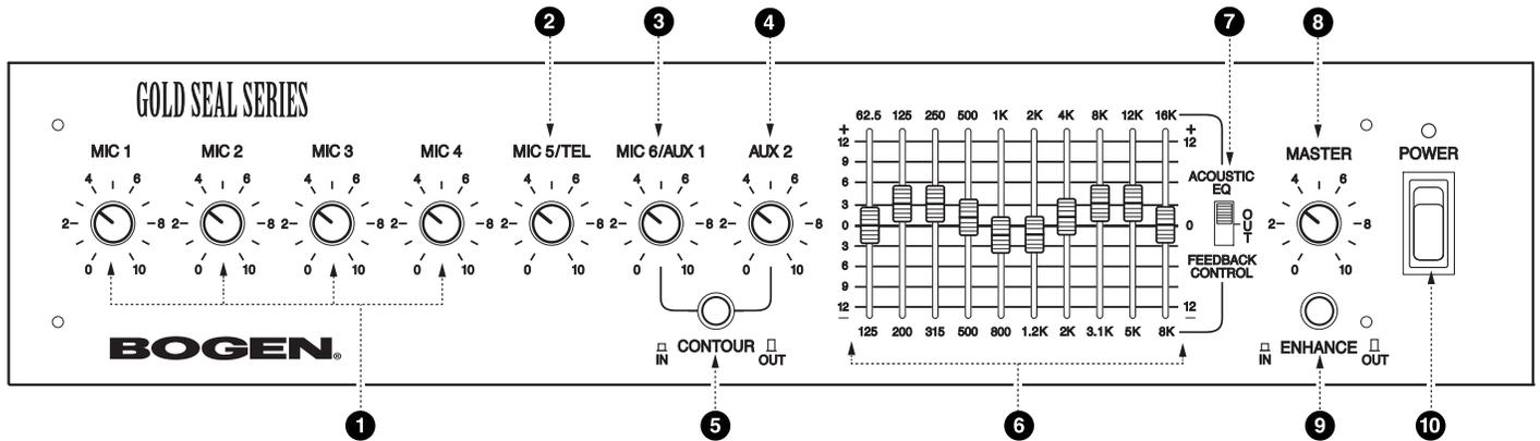
1. **MIC 1 to 4** - Individual level controls for dedicated microphone inputs.
