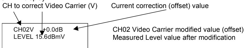
The displayed CH02V is the channel to be modified. The displayed mode is the video carrier. The calibration adjustment is applied to both the video carrier and audio carrier readings.
