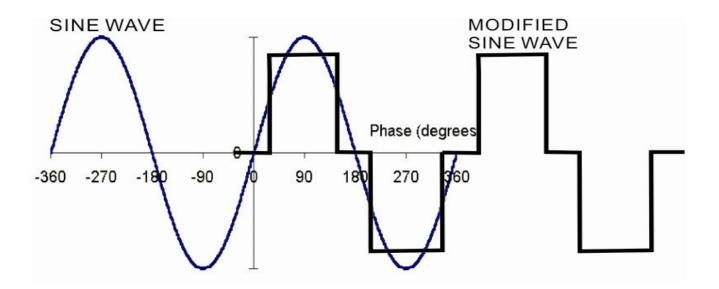
FIGURE 1: Modified Sine Wave and Sine Wave Comparison
