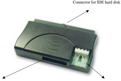
Connector for serial ATA cable
