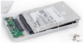
3. Use one hand to hold the drive and keep it from falling out of the bottom case, then flip the bottom case upside down to access the screw holes on the bottom. Use a Phillips screwdriver to install the two shorter machine-threaded screws in the screw holes circled in the picture below. This will secure the drive to the bottom case. When you have installed both screws, flip the bottom case back over.
