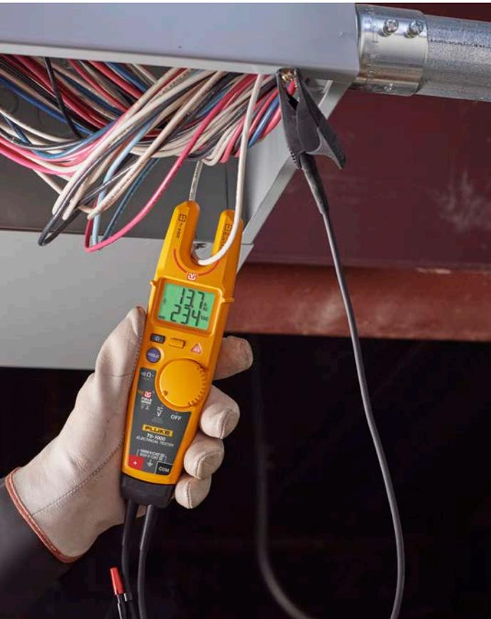
To measure ac voltage and ac current using FieldSense Technology:
