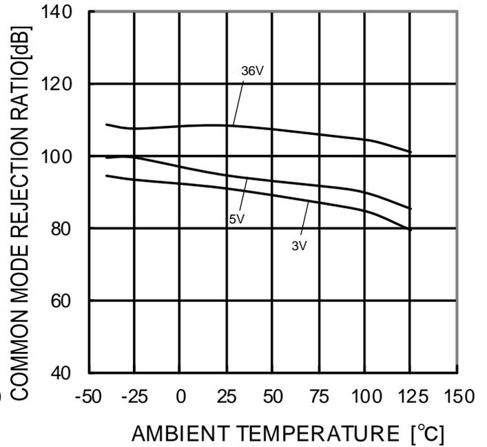
Figure 23. Common Mode Rejection Ratio vs Ambient Temperature (V<sub>OUT</sub>=1.4V)
