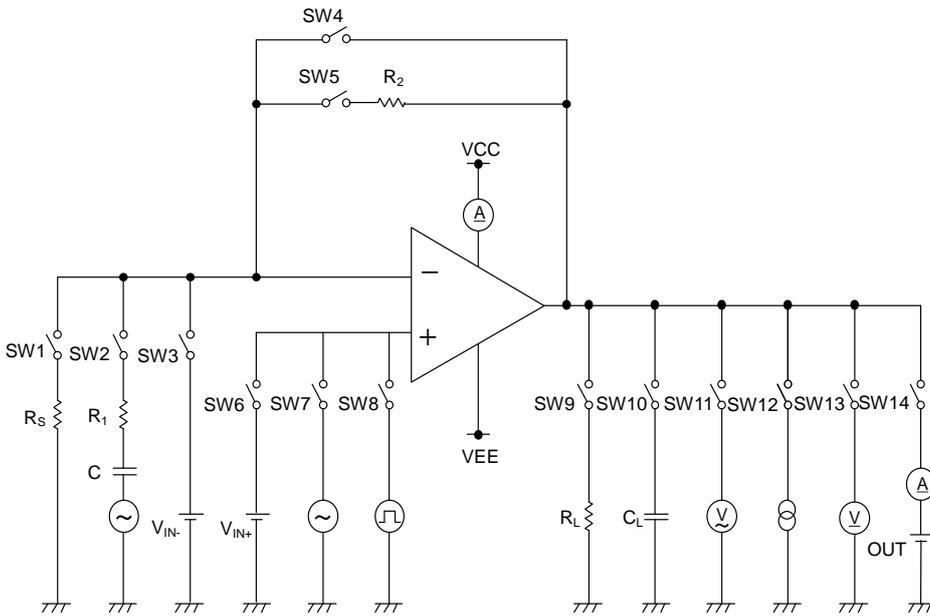
Figure 49. Test Circuit 2 (One Channel Only)
