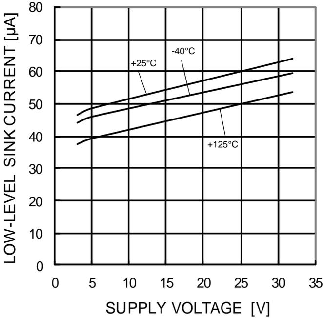
Figure 33. Low Level Sink Current vs Supply Voltage ( $V_{OUT}=0.2V$ )
