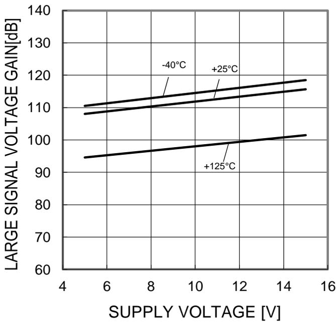
Figure 43. Large Signal Voltage Gain vs Supply Voltage
