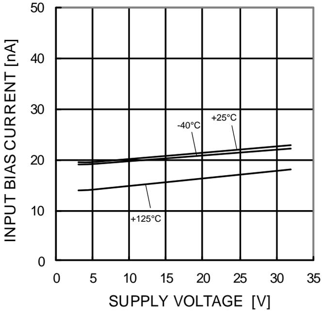
Figure 37. Input Bias Current vs Supply Voltage
