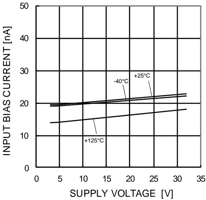
Figure 14. Input Bias Current vs Supply Voltage ( $V_{ICM}=0V$ ,  $V_{OUT}=1.4V$ )
