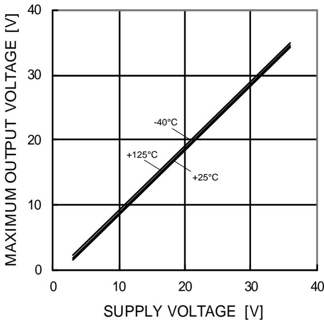
Figure 27. Maximum Output Voltage vs Supply Voltage (R<sub>L</sub>=10kΩ)
