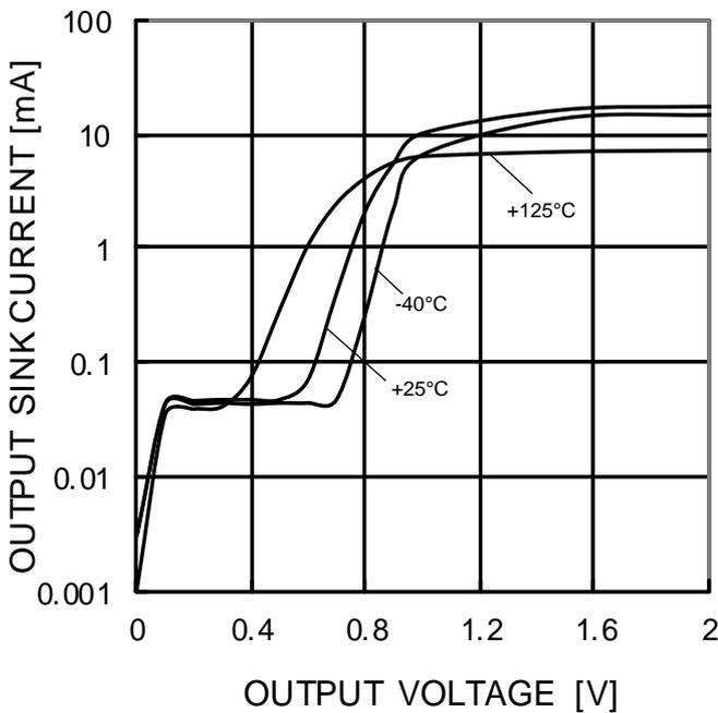
Figure 31. Output Sink Current vs Output Voltage (V<sub>CC</sub>=5V)
