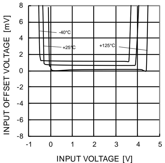
Figure 17. Input Offset Voltage vs Input Voltage ( $V_{CC}=5V$ )
