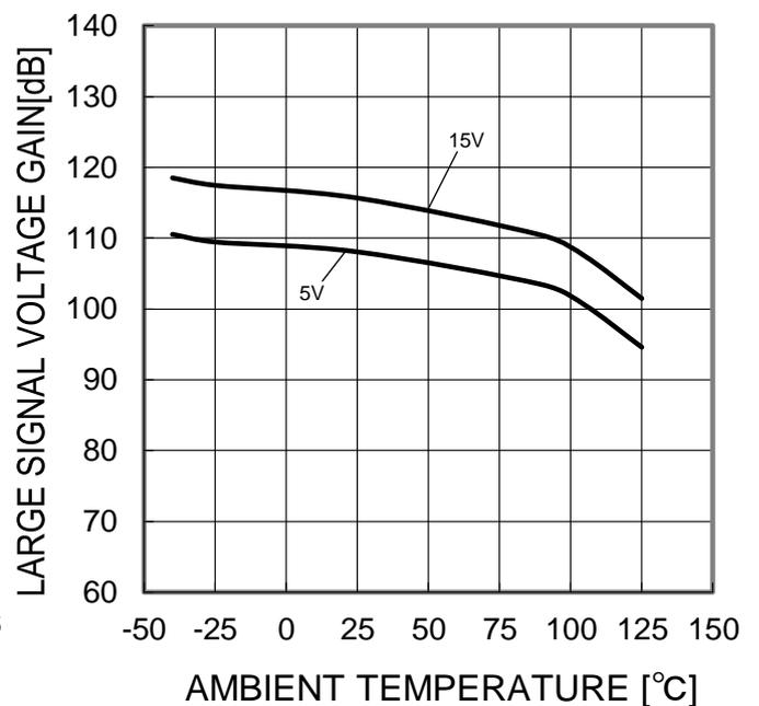
Figure 44. Large Signal Voltage Gain vs Ambient Temperature
