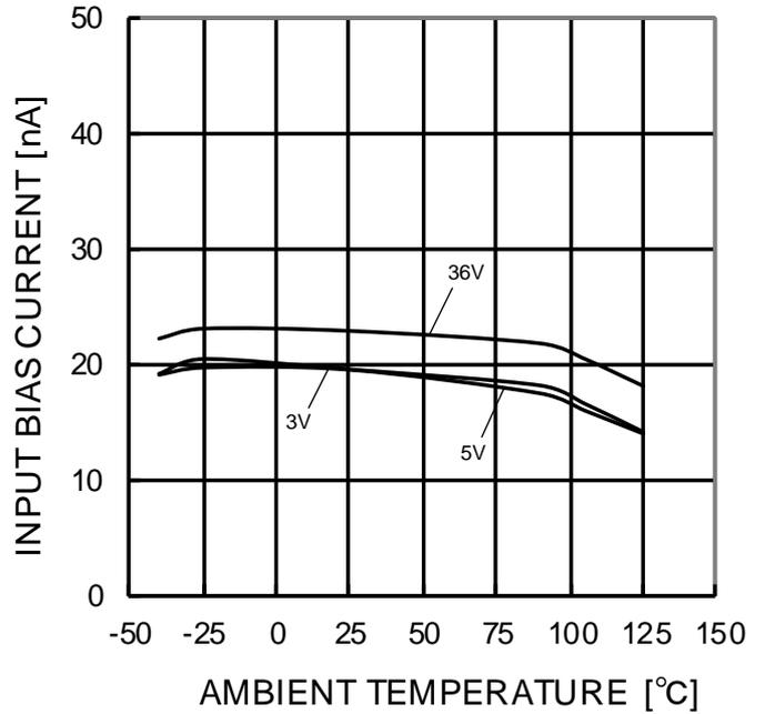
Figure 38. Input Bias Current vs Ambient Temperature
