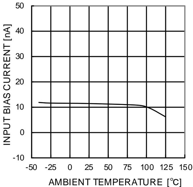
Figure 16. Input Bias Current vs Ambient Temperature ( $V_{CC}=30V$ ,  $V_{ICM}=28V$ ,  $V_{OUT}=1.4V$ )
