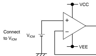
Figure 56. Example of application circuit for unused op-amp
