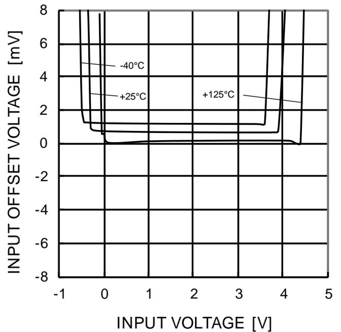
Figure 40. Input Offset Voltage vs Input Voltage
