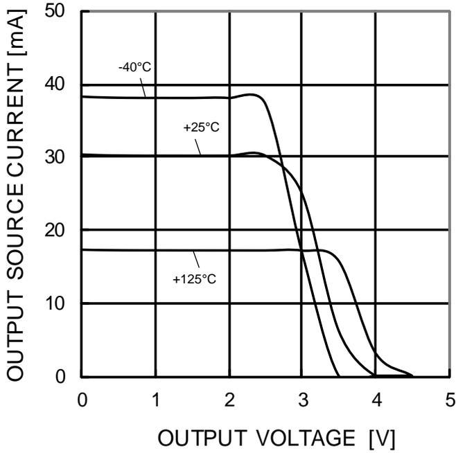
Figure 29. Output Source Current vs Output Voltage (V<sub>CC</sub>=5V)
