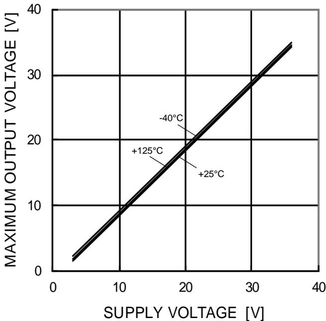
Figure 4. Maximum Output Voltage vs Supply Voltage (R<sub>L</sub>=10kΩ)
