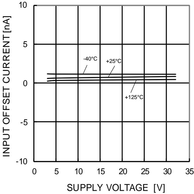
Figure 18. Input Offset Current vs Supply Voltage
