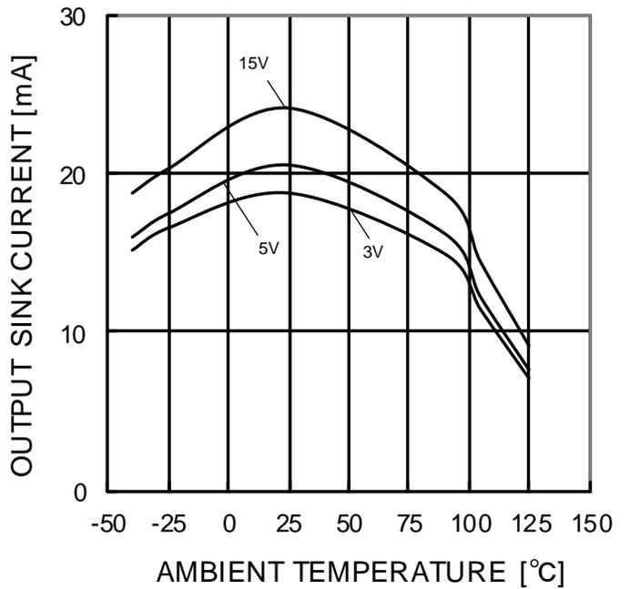
Figure 32. Output Sink Current vs Ambient Temperature (V<sub>OUT</sub>=V<sub>CC</sub>)
