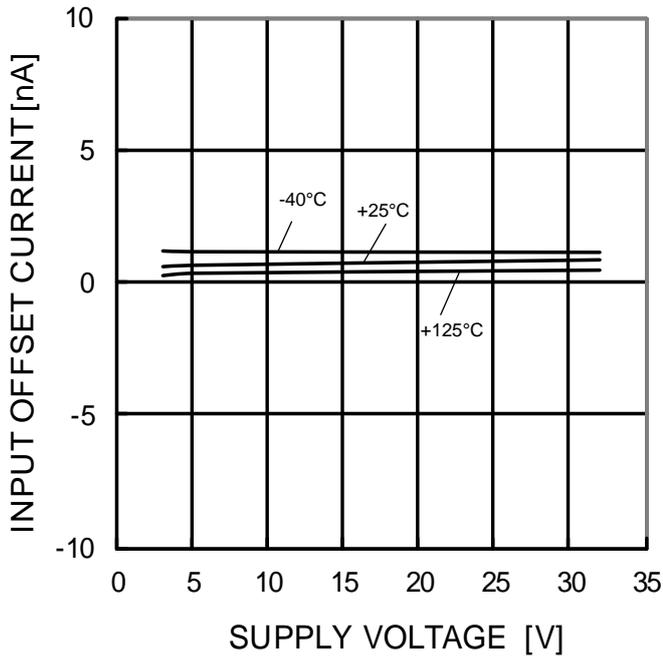
Figure 41. Input Offset Current vs Supply Voltage
