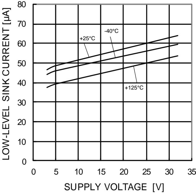
Figure 10. Low Level Sink Current vs Supply Voltage ( $V_{OUT}=0.2V$ )
