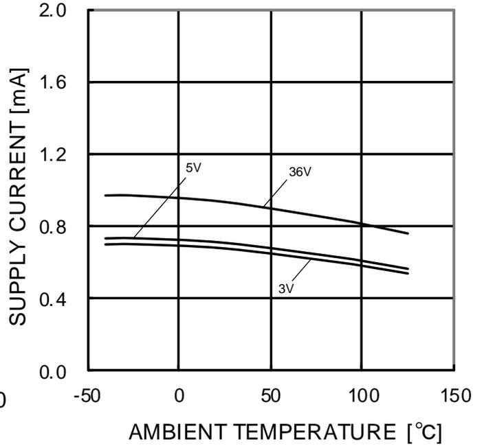
Figure 26. Supply Current vs Ambient Temperature
