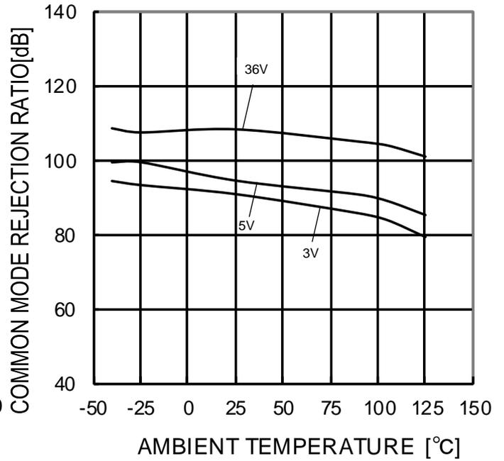
Figure 46. Common Mode Rejection Ratio vs Ambient Temperature (V<sub>OUT</sub>=1.4V)
