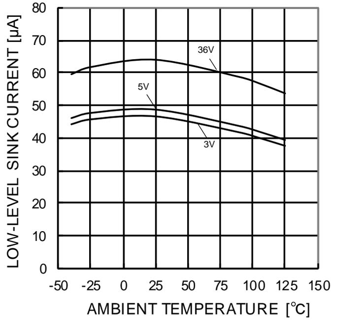
Figure 11. Low Level Sink Current vs Ambient Temperature ( $V_{OUT}=0.2V$ )
