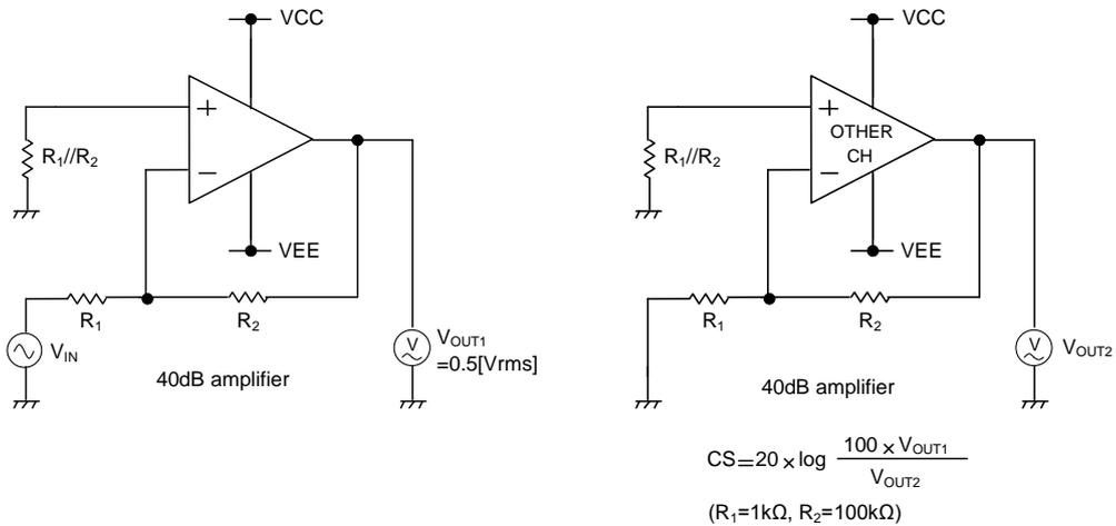
Figure 51. Test Circuit 3 (Channel Separation)
