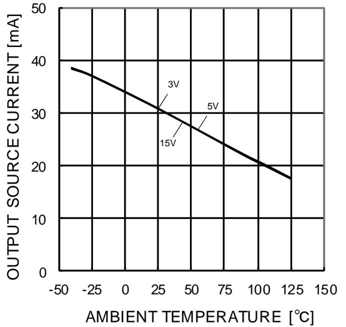
Figure 30. Output Source Current vs Ambient Temperature (V<sub>OUT</sub>=0V)
