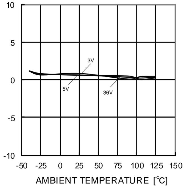
Figure 42. Input Offset Current vs Ambient Temperature
