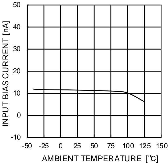
Figure 39. Input Bias Current vs Ambient Temperature
