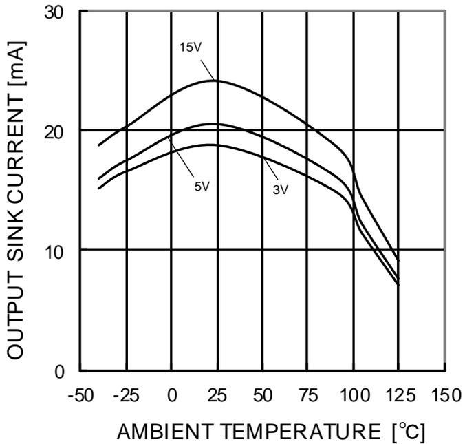
Figure 9. Output Sink Current vs Ambient Temperature (V<sub>OUT</sub>=V<sub>CC</sub>)
