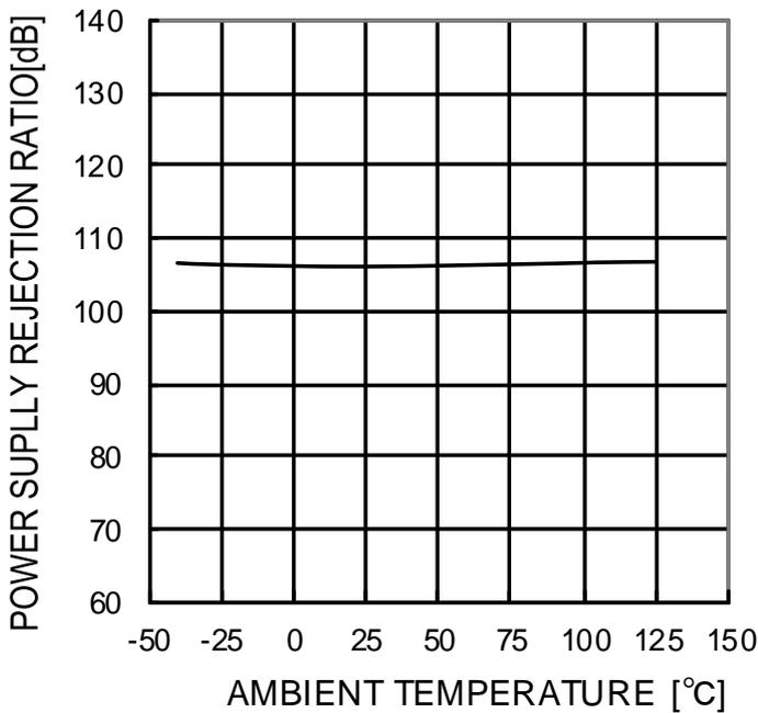
Figure 24. Power Supply Rejection Ratio vs Ambient Temperature
