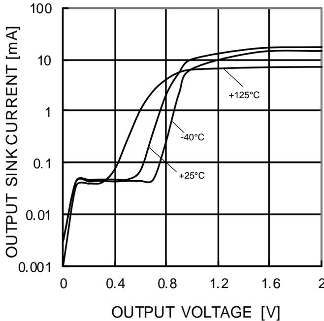
Figure 8. Output Sink Current vs Output Voltage (V<sub>CC</sub>=5V)
