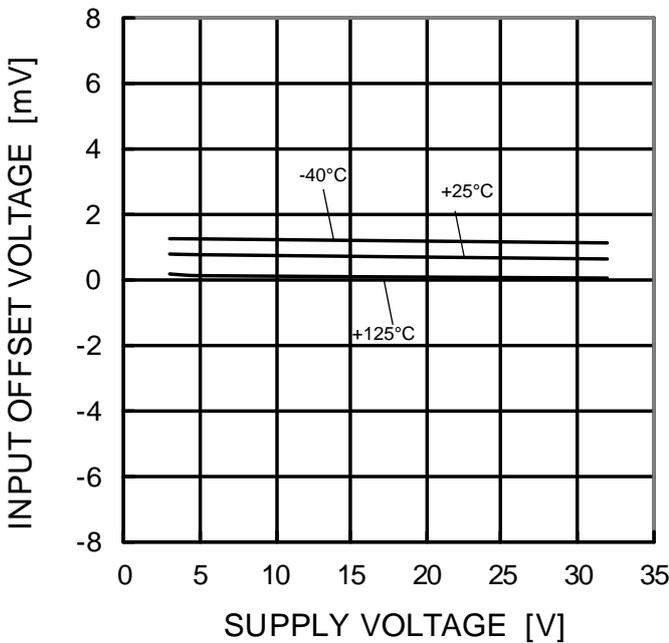
Figure 35. Input Offset Voltage vs Supply Voltage ( $V_{ICM}=0V, V_{OUT}=1.4V$ )
