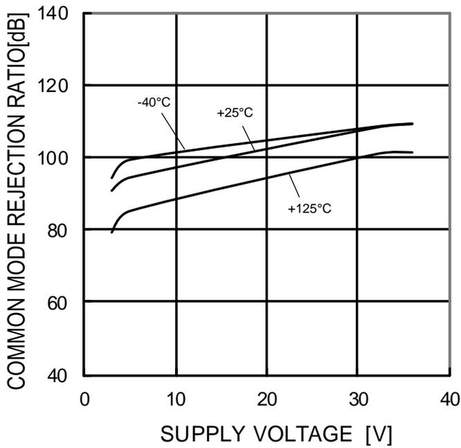
Figure 22. Common Mode Rejection Ratio vs Supply Voltage (V<sub>OUT</sub>=1.4V)
