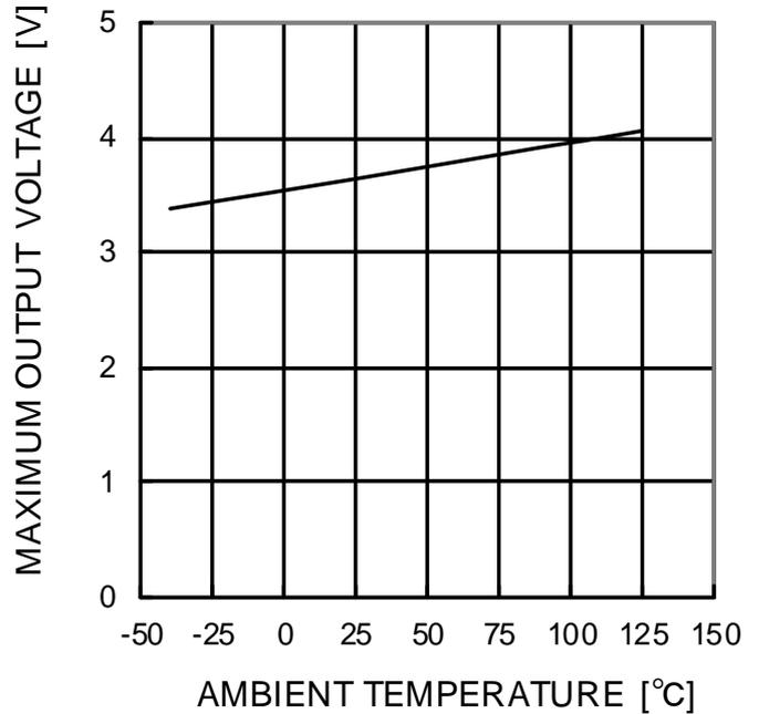
Figure 28. Maximum Output Voltage vs Ambient Temperature (V<sub>CC</sub>=5V, R<sub>L</sub>=2kΩ)
