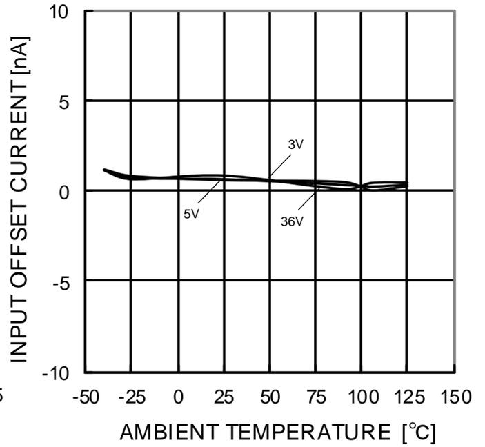
Figure 19. Input Offset Current vs Ambient Temperature
