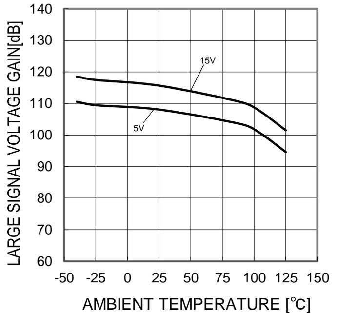
Figure 21. Large Signal Voltage Gain vs Ambient Temperature
