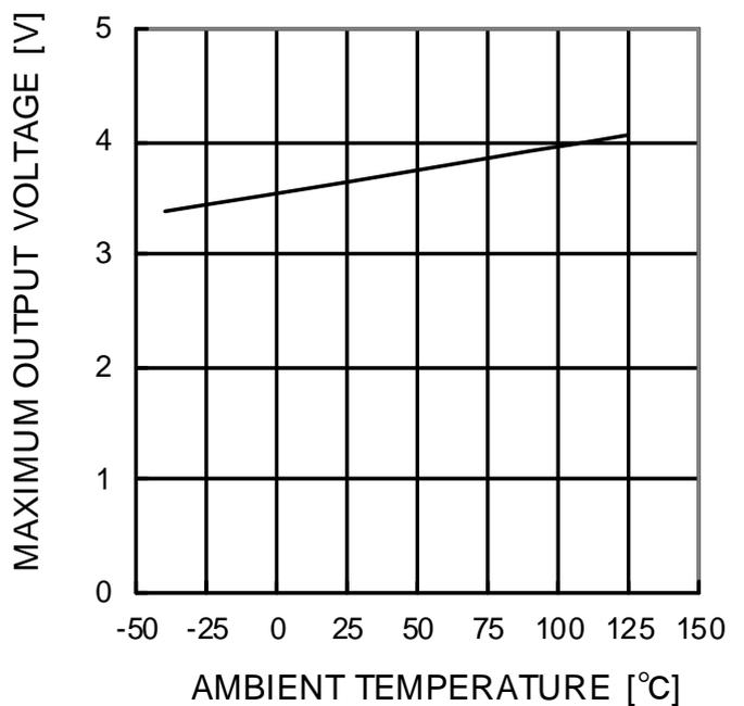
Figure 5. Maximum Output Voltage vs Ambient Temperature (V<sub>CC</sub>=5V, R<sub>L</sub>=2kΩ)
