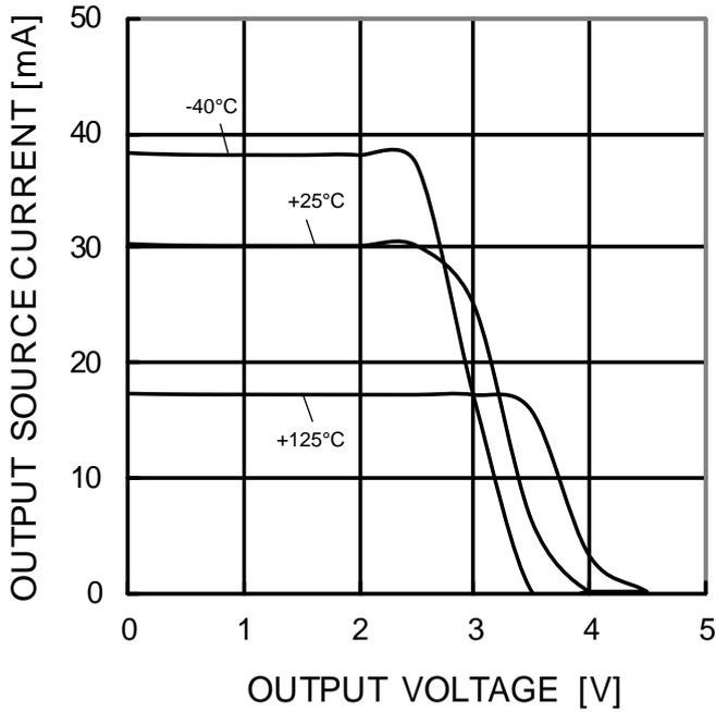
Figure 6. Output Source Current vs Output Voltage (V<sub>CC</sub>=5V)
