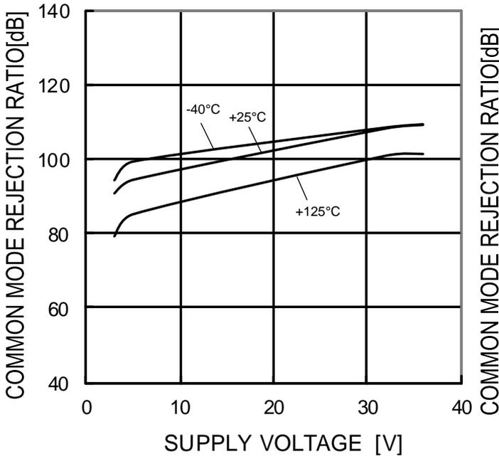
Figure 45. Common Mode Rejection Ratio vs Supply Voltage (V<sub>OUT</sub>=1.4V)
