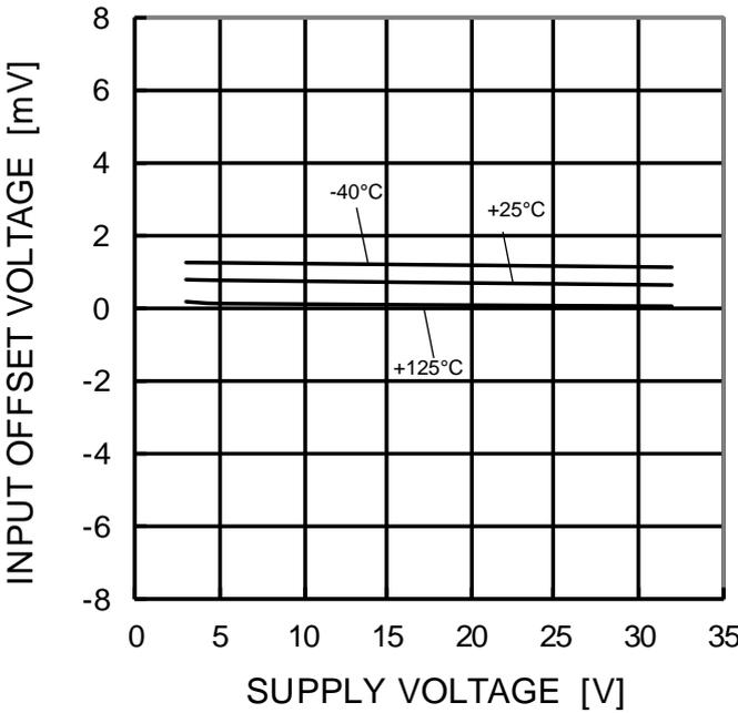
Figure 12. Input Offset Voltage vs Supply Voltage ( $V_{ICM}=0V, V_{OUT}=1.4V$ )
