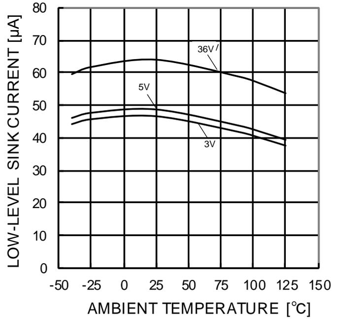
Figure 34. Low Level Sink Current vs Ambient Temperature ( $V_{OUT}=0.2V$ )
