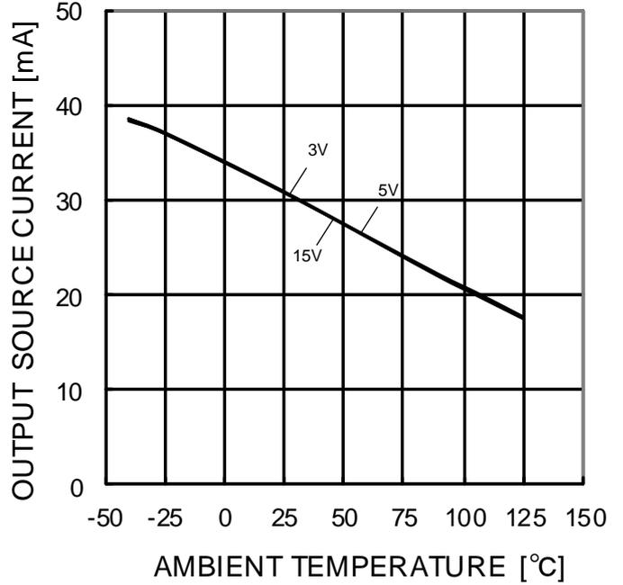
Figure 7. Output Source Current vs Ambient Temperature (V<sub>OUT</sub>=0V)
