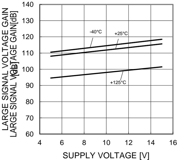
Figure 20. Large Signal Voltage Gain vs Supply Voltage
