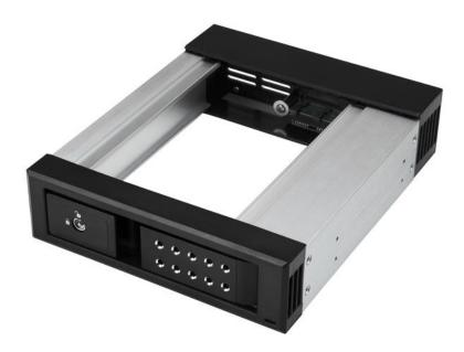
This removable hard drive hot-swap bay makes it easy to swap 3.5" SATA or SAS drives in and out of your server or desktop computer, using an available 5.25" front drive bay. It features a trayless design that saves you installation time and enables you to insert or remove drives as needed, creating a convenient solution for drive maintenance and interchangeability of data between multiple systems.
