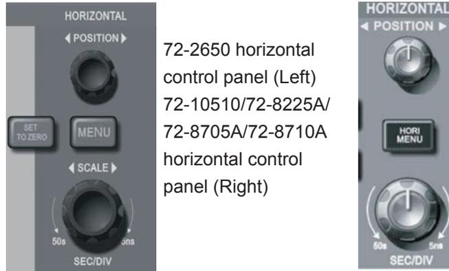
Figure 1-10 Horizontal Control Area on the Panel
