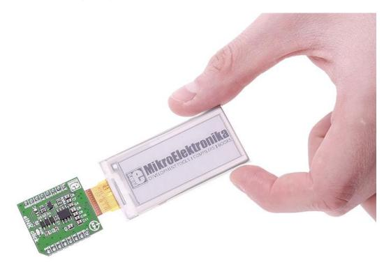
The display uses electronic ink, which makes the display "Bistable". It means that the display consumes power only when something is changing on the screen. This reduces the power consumption of the target device considerably. So, the display retains the image even when the power is off.
