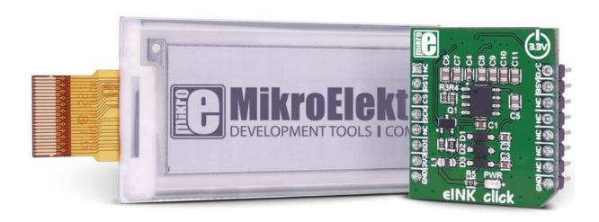
eINK click is an adapter for connecting eINK displays, with a 24pin ribbon cable.
