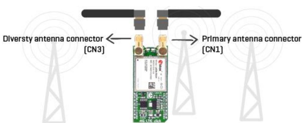
A diversity antenna only covers the Rx frequencies, and its job is to acquire an independent sample of data. The application in which you are using the click board can then choose the receive signal it wants to use.
