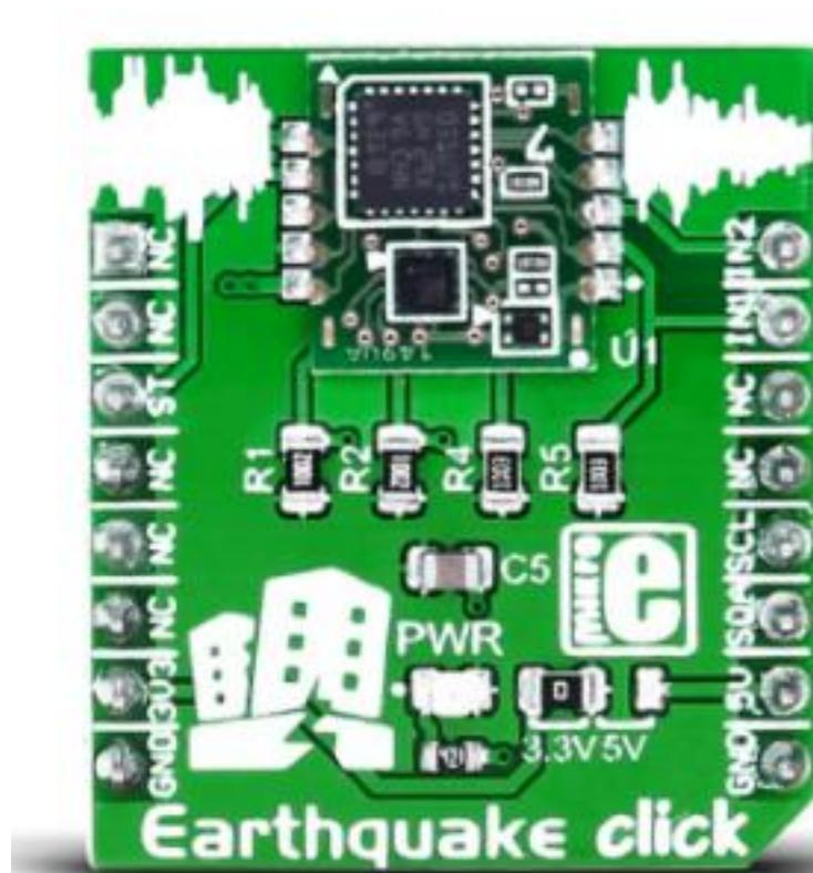
**Earthquake click** carries [D7S](#), the world's smallest high-precision seismic sensor from Omron.
