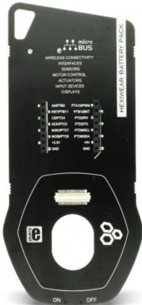
**Hexiwear Battery Pack** will keep your favorite IoT development kit charged. You can add any functionality with the onboard mikroBUS™ socket. Add sensors, transceivers, speech recognition modules and more. No more cables and worrying if the battery on it will last the day.
