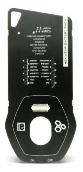
**Hexiwear Battery Pack** will keep your favorite IoT development kit charged. You can add any functionality with the onboard mikroBUS<sup>™</sup> socket. Add sensors, transceivers, speech recognition modules and more. No more cables and worrying if the battery on it will last the day.
