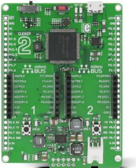
**Clicker 2 for MSP432** is a compact development board with two mikroBUS™ sockets for click board connectivity. It carries the SimpleLink™ [MSP432™](#) - ARM® 32-Bit Cortex®-M4F CPU with integrated 1MSPs 14-bit SAR-based ADC from **Texas Instruments**.
