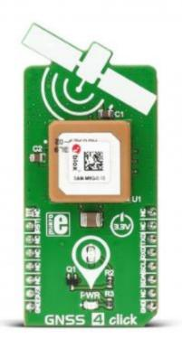
**GNSS 4 click** carries <u>SAM-M8Q</u> patch antenna module from u-blox.
