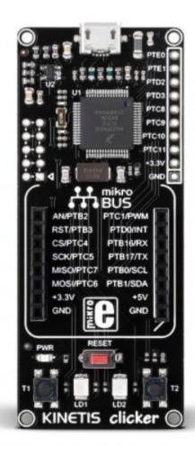
**Kinetis clicker** is an amazingly compact starter development kit which brings click board connectivity an NXP's Kinetis ARM Cortex<sup>™</sup>-M4 microcontroller.
