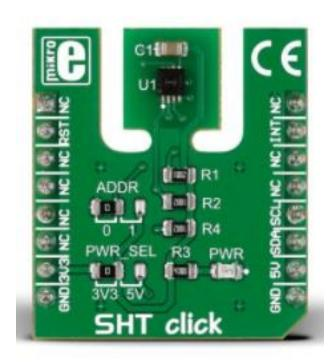
SHT click is a temperature and humidity sensing click board that carries Sensiron's <u>SHT3x-DIS</u> IC. Compared to its predecessor (SHT11), SHT3x click has increased reliability and enhanced signal processing features with a high signal-to-noise ratio.
