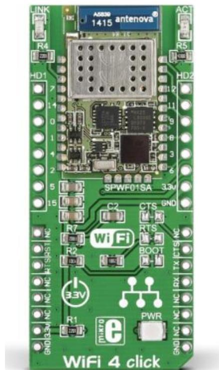
**WiFi 4 click** carries [SPWF01SA](#), a complete standalone WiFi module with a single-chip 802.11 b/g/n transceiver, a 32-bit STM32 MCU, along with a built-in 2.4 GHz ISM band antenna.
