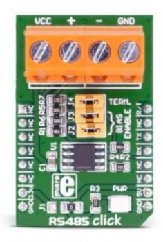
**RS485 click 5V** carries the <u>ADM485</u> differential line transceiver from Analog Devices. It is designed for balanced data transmission and complies with EIA standards RS-485 and RS-422.
