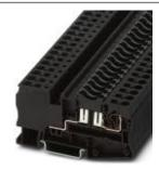
Fuse modular terminal block, fuse type: Flat, connection method: Spring-cage connection, cross section: 0.08 mm²- 6 mm², AWG: 28 - 10, nominal current: 30 A, nom. voltage: 400 V, width: 8.2 mm, fuse type: C, mounting type: NS 35/7,5, NS 35/15, color: black
