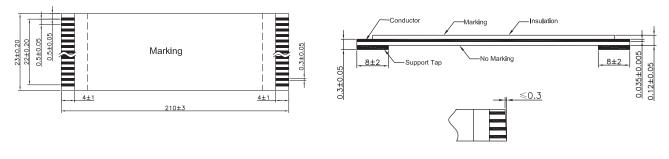
Dimensions : Millimetres Tolerances: ±0.3mm
