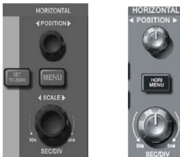
Figure 1-10 Horizontal Control Area on the Panel 72-7610 (Left) 72-10510 (Right)
