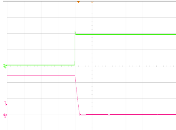
Figure 8: AVD85B-48S12 Output Voltage Shut Down By Remote Off V_{IN} = 48V_{dc} , I_O = I_{O,max} , 10mS/div Ch 2: Remote Off (2V/div) Ch 4: V_O (5V/div)
