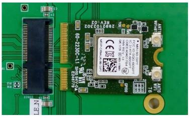
Connect the two antennas to the u.FL connectors on the DVK-ST60-2230C/ DVK-SU60-2230C board.
