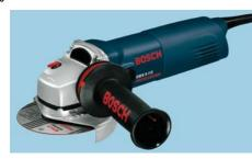
800W 115mm disc diameter angle grinder. Features tool-less guard adjustment automatically locks itself for protection. Direct motor cooling with special air ducting and ventilation vents on rear of tool.
