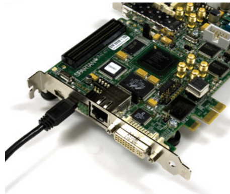
Figure 60: Connecting the USB Cable to the USB-JTAG Connector of the SP605 Board
