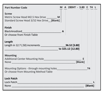
Part Number Code example: A280HT-4.80T4 Series 280HT Card-Lok five piece 121.9 (4.80) long with black anodize finish, 4-40 tapped hole for mounting.
