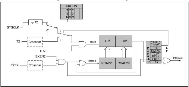
Figure 19.12. T2 Mode 1 Block Diagram
