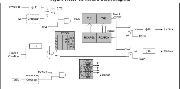
Figure 19.13. T2 Mode 2 Block Diagram
