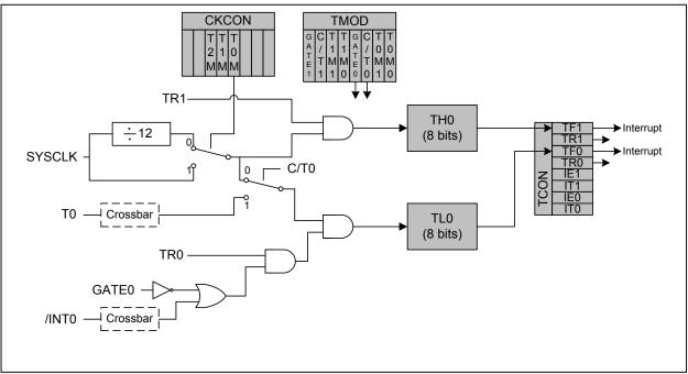
Figure 19.3. T0 Mode 3 Block Diagram
