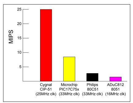
Figure 1.4. Comparison of Peak MCU Execution Speeds
