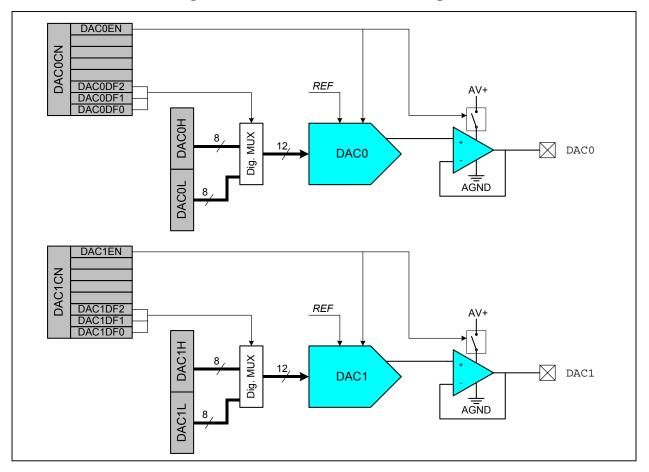
Figure 7.1. DAC Functional Block Diagram
