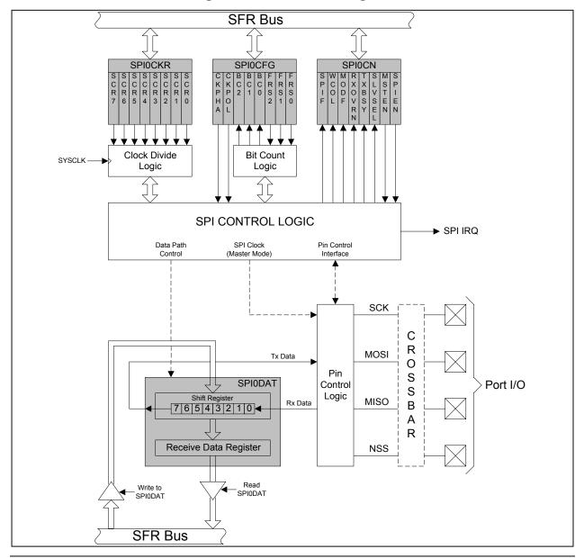
Figure 17.1. SPI Block Diagram
