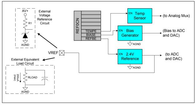
Figure 9.1. Voltage Reference Functional Block Diagram
