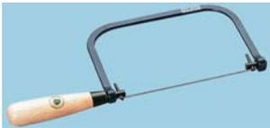
Correct tension is applied to the blade by turning the handle. The blade can be turned to cut at any angle. Depth of bow 120mm 4¾in.
