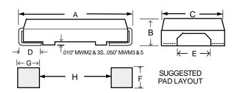
Exceptional perfomance and reliability is achieved via highest grade materials and processing. An all-welded wirewound construction is standard, featuring premium-grade wire for superior stability and surge capability. Opt. L low profile models feature a non-inductive metal plate element. The power film version (Opt.M) achieves values as high as  $1M\Omega$  and is inherently low inductance thereby enabling stable operation at high frequencies.
