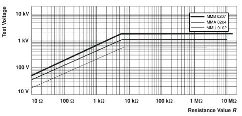
Pulse load rating in accordance with IEC 60115-1, 4.27; 10  $\mu s$  / 700  $\mu s$ ; 10 pulses at 1 minute intervals; for premissible resistance change 0.5 %
