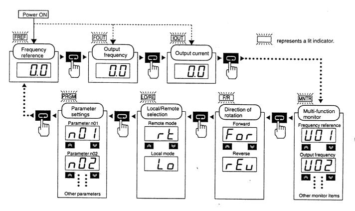
Note: If the power is turned OFF with the FOUT or IOUT indicator lit, the same indicator will light when the power is turned ON again. In other cases, the FREF indicator will light when the power is turned ON.
