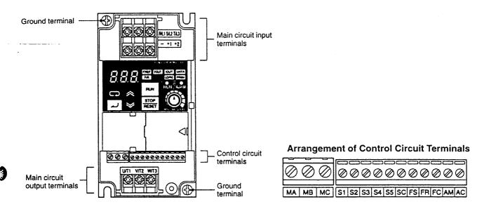
Note: This illustration shows the terminal block with the front cover removed.
