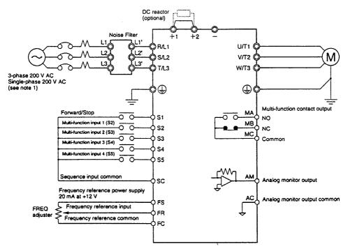
Note: 1. Connect single-phase 200 V AC to terminals R/L1 and S/L2 of the 3G3JV-AB ...
