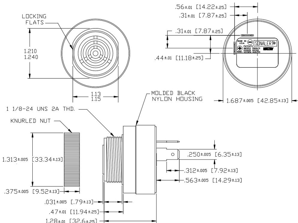
NOTE A: TERMINALS-.032 BRASS, TIN PLATED WITH .070 DIA. WIRE HOLE. WILL ACCEPT 1/4" QUICK CONNECT.
