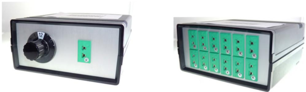
A 12-way selector in a moulded housing with aluminium front and rear panels. The 12 rear inputs are switched via a front mounted rotary selector switch to the single output socket. Internally wired with thermocouple compensating cable.
