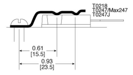
Hole Diameter for Screw: 4.2mm
