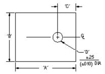
Thermasil III electrically insulating pad with adhesive backing for a TO-220 device. Composed of a silicone elastomer binder with thermally conductive filler and reinforced with finely woven glass cloth to resist tearing.
