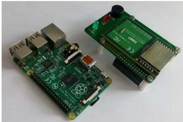
**Figure 26: NFC Controller and Raspberry Pi Boards**
