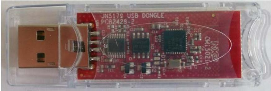
Figure 24: JN5179 USB Dongle
